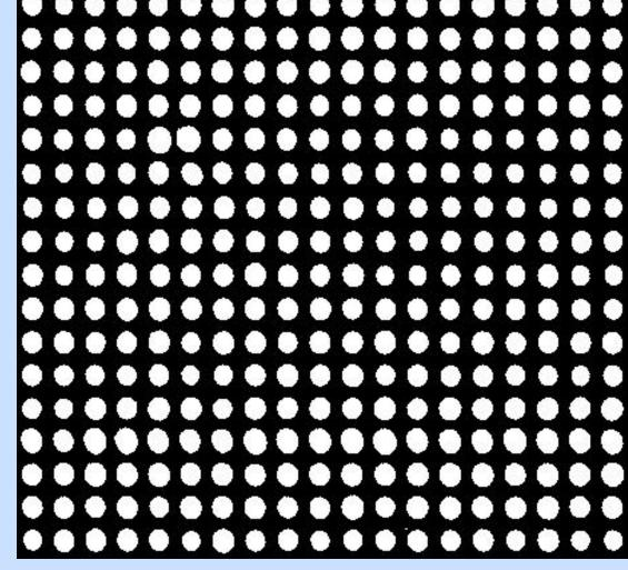
Figure 1 shows the concept of pre-patterned media where each bump is an isolated magnetic dot. When such media are replicated (e.g. by nanoimprint), any errors on the master are copied. The size, shape and position of the bumps must be measured and then controlled in order to achieve low noise recording and playback.
