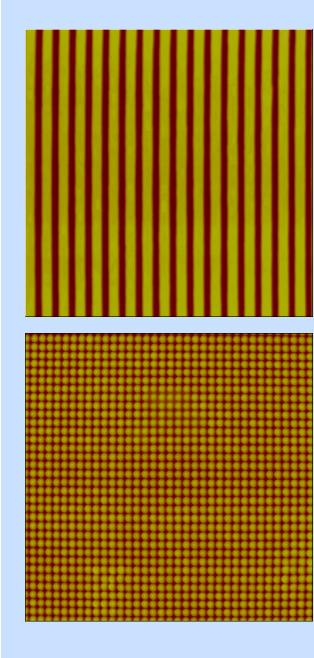
Fig. 2 Calibration standard: 292-nm pitch, 1-D holographic grating of Ti lines on Si. Mean pitch = 292.096  $\pm$  0.015nm (measured at PTB)
