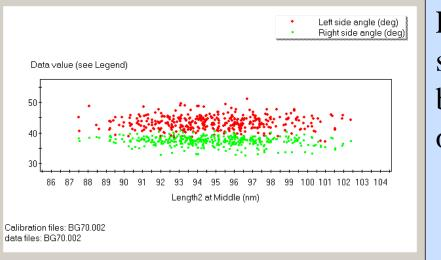
Fig. 10. This chart directly shows that the side wall angles did not correlate with bump length, remaining relatively constant over the range of feature lengths.
