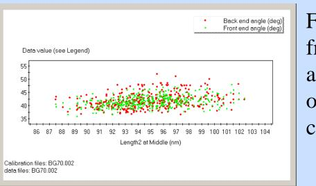
Fig. 11. As with left and right angles, the front and back angles remained approximately constant with feature length, or perhaps increased slightly.This slight correlation is probably not significant.
